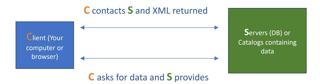
Web services work on a network and allow data to be exchanged. They use standards (OGC) to maximize interoperability.
